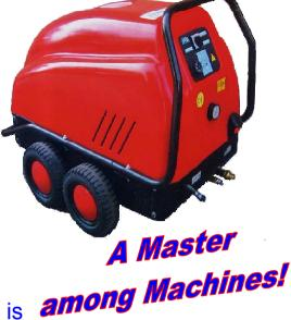
adjustable from 30 to 110 degrees centigrade. The traditional horizontal pump contains three hard wearing ceramic pistons and it is direct coupled to a three phase, air cooled electric motor. The water is heated as it passes through the double steel coil of the vertical boiler unit
