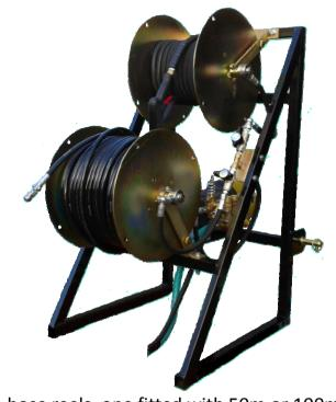
Two hose reels, one fitted with 50m or 100m of thermoplastic drain jetting hose (maximum capacity 100m of this hose), the other fitted with 30m or 50m of high pressure hose and lance for general use.
